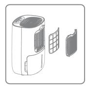
The filter can either be cleaned using a vacuum cleaner or in warm, soapy water below 40°C. Make sure that the filter is completely dry before reinserting back into the dehumidifier.
